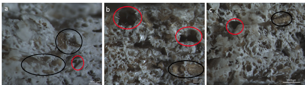
Fig. 3. Microscopic images for the cross-sections of broken tensile test specimens of various PPHF composites a) 5% Hemp PP, b) 10% Hemp PP and c) 20% Hemp PP. Black circles show fibers and red circles represent porosities. (For interpretation of the references to colour in this figure legend, the reader is referred to the Web version of this article.)
