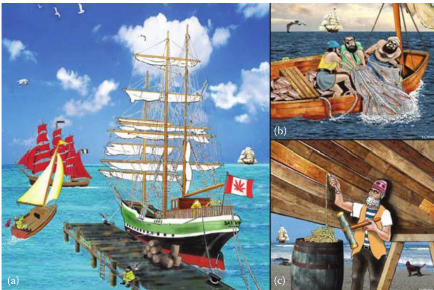
FIGURE 7.4 Major maritime uses of hemp in the past. Hemp was used for (a) sails, ropes, and rigging, (b) nets, and (c) oakum for caulking seams in wooden ships, and was indispensable for navies. Prepared by B. Flahey.
