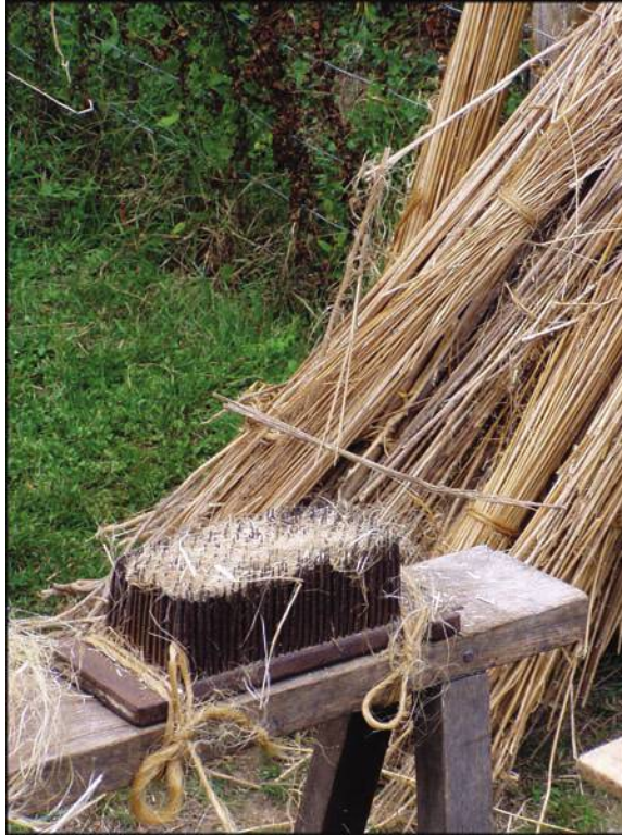
FIGURE 7.20 A hackle employed for aligning and cleaning raw hemp fiber. In general, hackles are combs or boards with long steel teeth for dressing fiber plants. Photo by CVB (CC BY SA 3.0).
