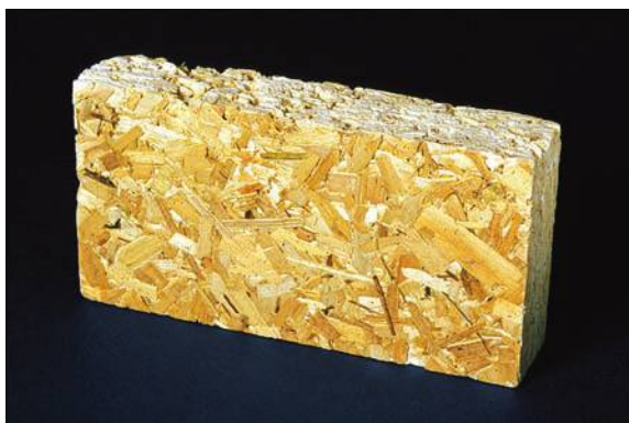
FIGURE 7.30 Fiberboard sample made with hemp. Photo by E. Small, sample supplied by K. Domier, University of Alberta, Edmonton.
