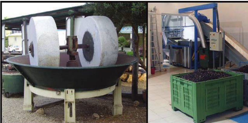
FIGURE 8.7 Examples of simple and complex edible vegetable oil extraction systems. Left: A simple, grinding wheel oil press. Photo by Avishai Teicher (CC BY 2.5). Right: A complex vegetable oil extraction factory. Photo by Bracodbk (CC BY 3.0).
