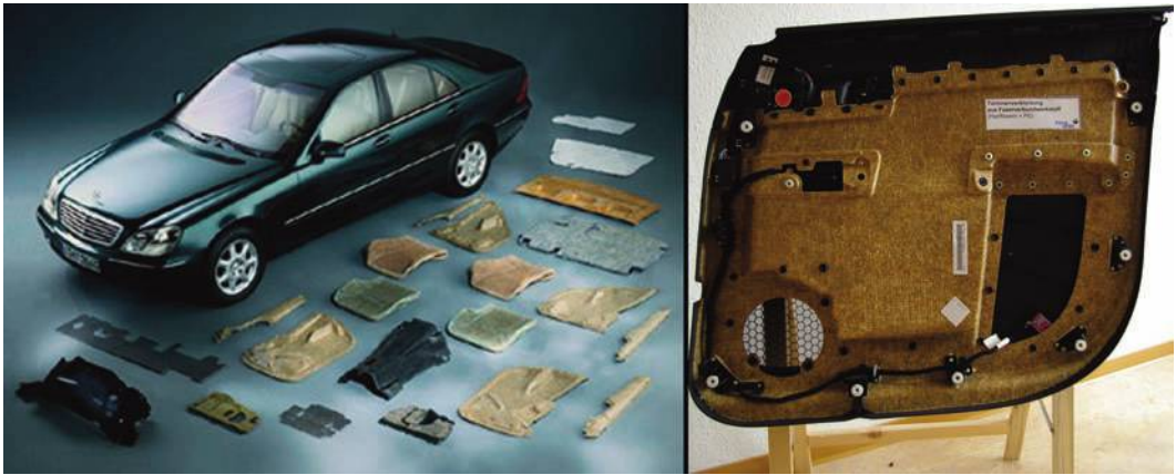
FIGURE 7.27 Molded and pressed fiber products. Left: C-class Mercedes-Benz automobiles have more than 30 parts made of natural fibers, including hemp. (Courtesy of Daimler.) Right: Interior carpeting of a car door made with a biocomposite of hemp fiber and polyethylene. Photo by Christian Gahle, Nova-Institut GmbH (CC BY SA 3.0).
