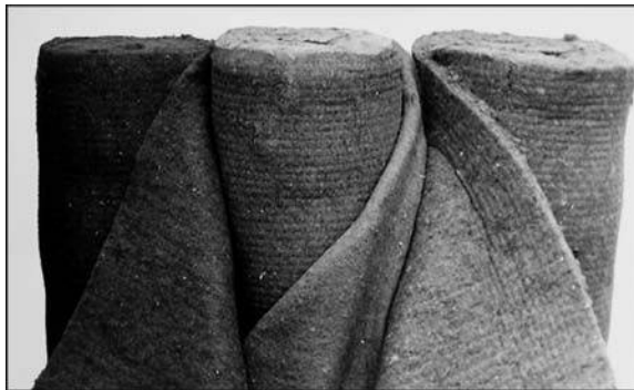
FIGURE 7.25 Multipurpose, nonwoven matting, fabricated from hemp. (Photo by E. Small, sample provided by Kenex Ltd., Pain Court, Ontario.)
